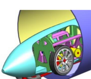
Assembled for the proposed flat floor tube. The guide wheels would have limited speed, and cornering would be restricted by side-load problems.
