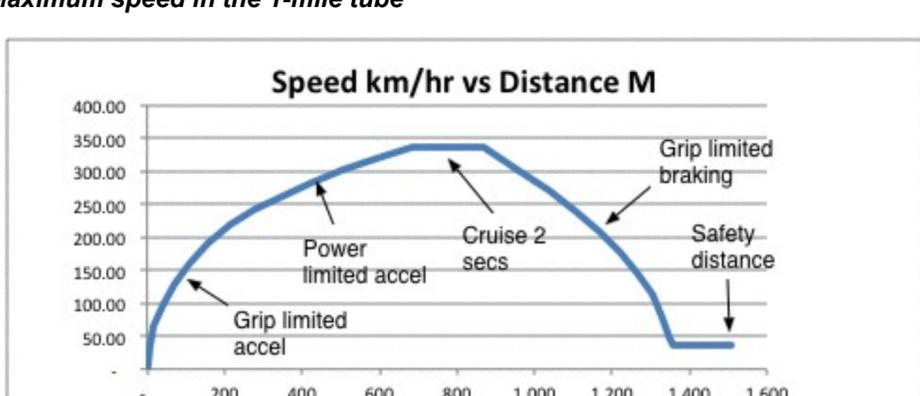
The tires should have a reliable friction coefficient of 1.0, soft racing tires go up to 1.4. The chart shows a 0.9g acceleration, a 2 second cruise, and 0.9g braking, the maximum speed for the 1-mile tube is 208 mph, 335 km/hr. This is conservative, and allows for a 250m braking safety margin before the end of the tube. 250 mph, 400 km/hr is possible with soft racing tires.
